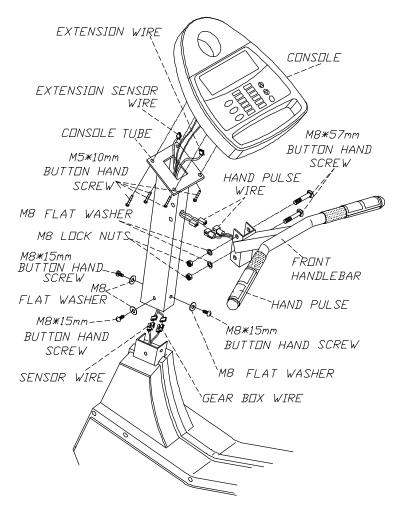
**7.** Attach wires in main frame to those in the console tube then secure console tube to main frame.
